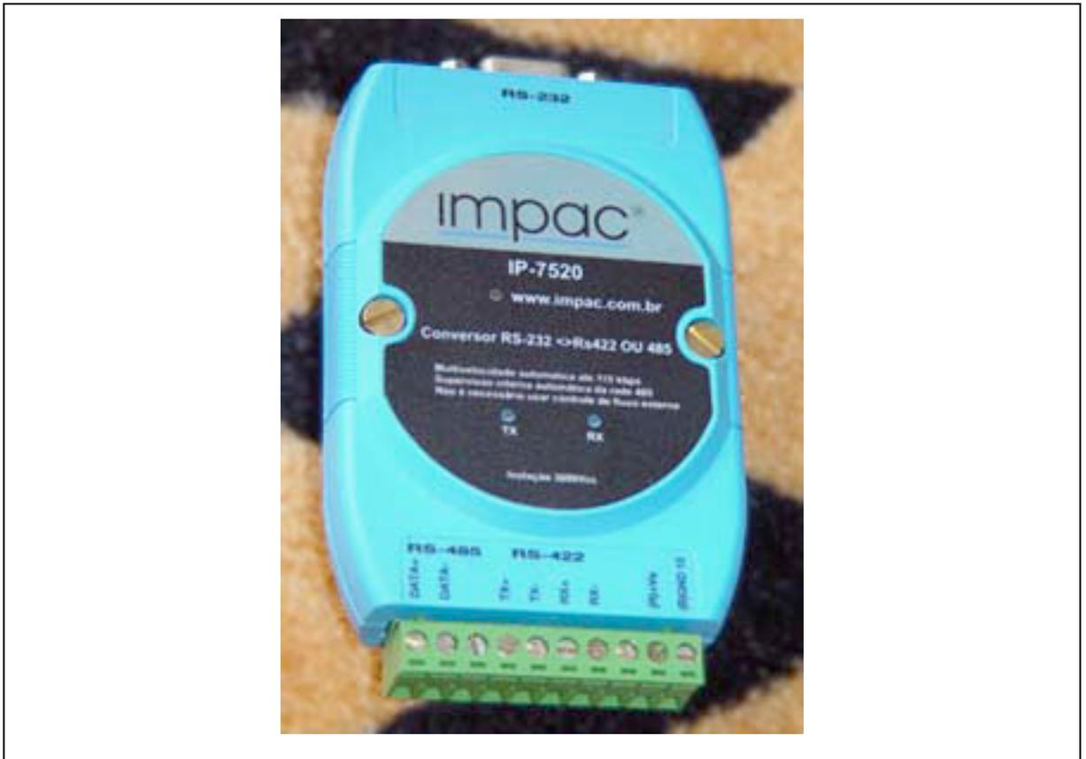
Figura 4. Conversor Serial RS232/422/485.
