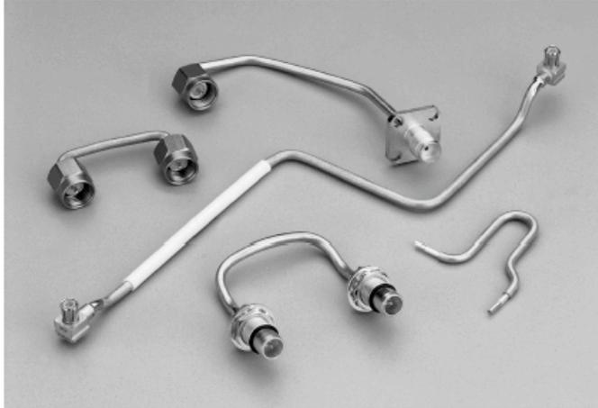
.086 diameter is the most common size Semi-Rigid cable. This size matches well with miniature high frequency connectors such as 2.4mm and SMP. The use of an aluminum jacket will allow final shaping at the installation site. Florida RF Labs® cable assemblies are Space Qualified and available unbent or shaped to your specifications.
