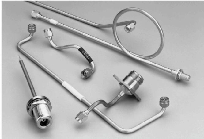
Semi-Rigid 141 offers high performance to 35 GHz with moderate insertion loss. The .141 diameter size cable matches well with high frequency connectors such as 2.9mm, BMA and SMA connectors. Florida RF Labs® offers Space Qualified assemblies bent to your specifications with a wide range of connectors.
