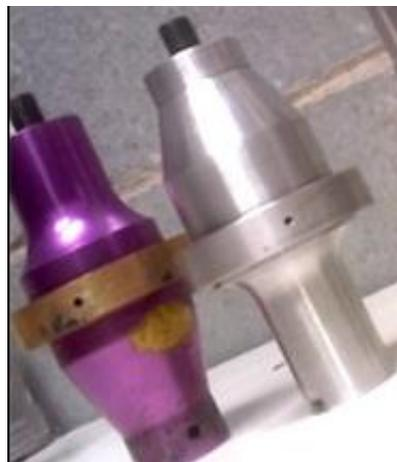
Figura 13 – TA's roxo e prata de 20 kHz (GNULTRASÔNICA, 2010)
