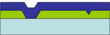
5- Deposition of polysilicon - the cantilever material
