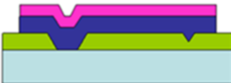
7- Etching the polysilicon - defining the cantilever
