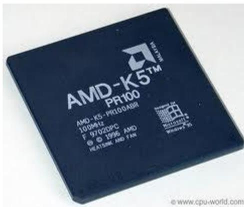
Figura 26: Processador K5. (Fonte: <http://www.cpu-world.com/CPUs/K5/>)
